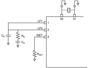
The external crystal devices and loop filter components should be kept close to the device. Loop filter and crystal PCB connection traces should be kept short and well separated from each other and from other signal traces. Other signal traces should not run underneath the device, the loop filter or crystal components.
