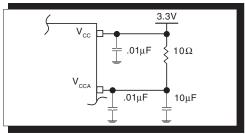
FIGURE 2. POWER SUPPLY FILTERING
