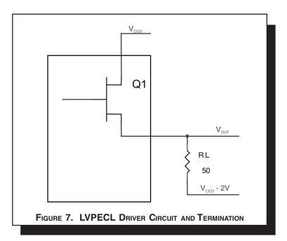
To calculate worst case power dissipation into the load, use the following equations which assume a 50 $\Omega$  load, and a termination voltage of V  $_{CCO}$  - 2V.
