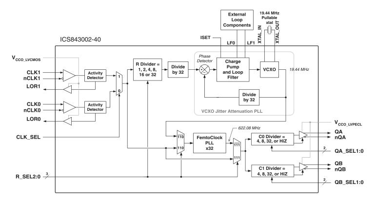
NOTE 1: 19.44MHz VCXO crystal shown is typical for SONET/SDH device applications.
